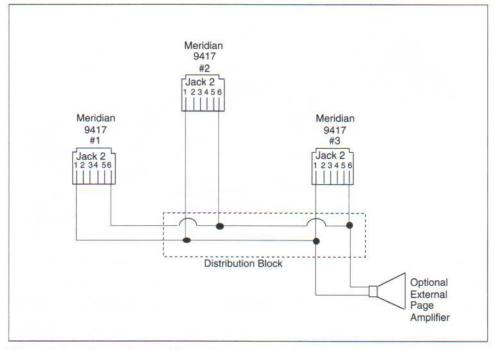
**Note**: A 6 conductor line cord is required to connect page lines. This cable is not supplied with the Meridian 9417 telephone. Contact your telephone representative or Telecom manager to have page lines connected to your telephones.
