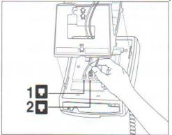
Attach line cord in jack 1 as shown by 1 . Attach the second line cord in jack 2 as shown by 2 .
