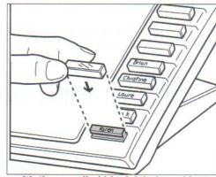
After programming the memory keys, label them with the supplied blank labels and key caps.<sup>†</sup>
