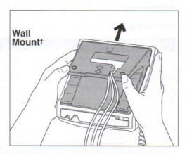
Slide the stand back until it clicks into the locked position, as shown in the desk or wall mount illustration above. The excess line cord fits into the stand of the telephone.
