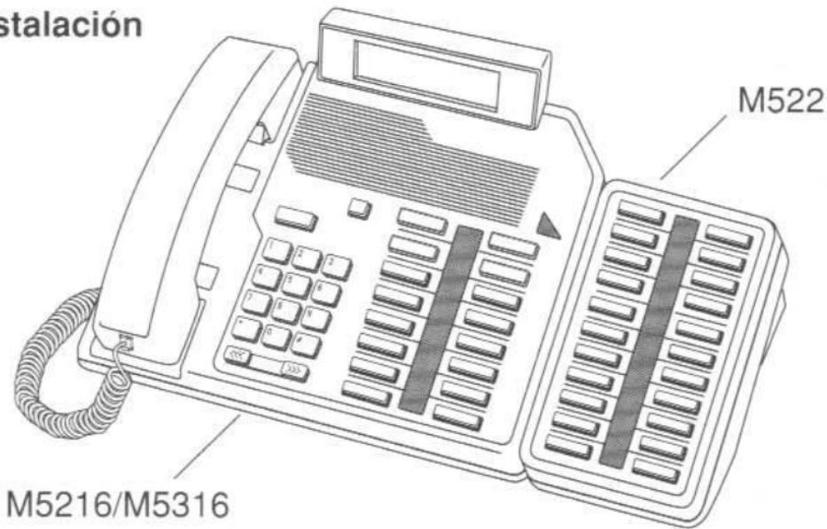
The M522 Add-On Module can be attached to the M5216 or M5316 Meridian Business Set to provide extra feature/line keys. When one M522 is connected, 22 additional feature/line keys are available to the Meridian Business Set. If required, you can also connect another M522 Add-On Module to increase the number of additional feature/line keys to 44.
