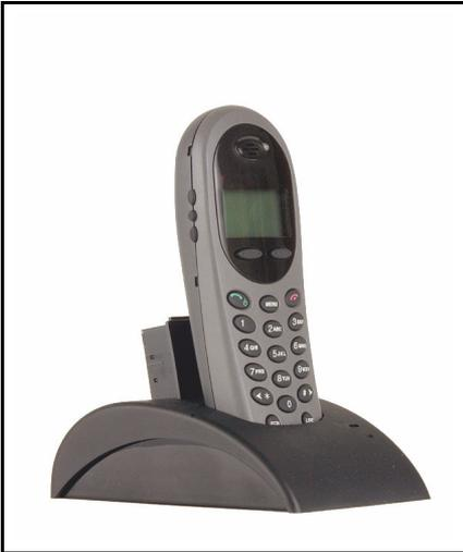
The Dual Charger comes with the appropriate power supply for the site. Place the Dual Charger on a flat, horizontal surface. Plug the power supply into the Dual Charger and into an appropriate wall outlet.
