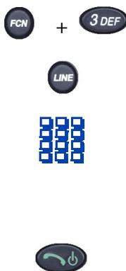
1. Press the **Function** key and the number **3** key to enter the active (idle) state.
